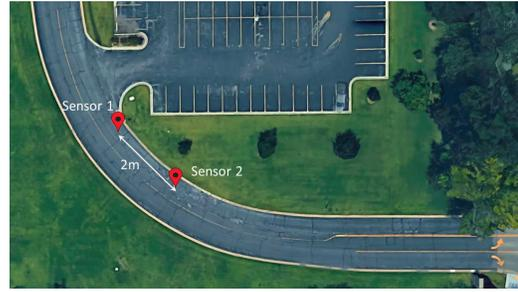
Fig. 13. Sensor setup on the entrance of campus.
