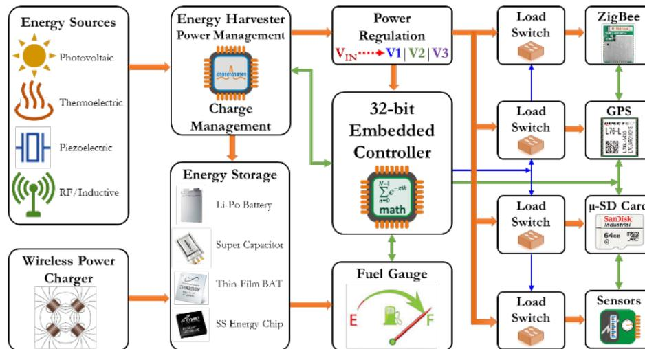
Figure 4. Overview of the system components [7].
