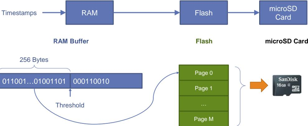
**Figure 16. Block diagram illustrating data buffering technique.**
