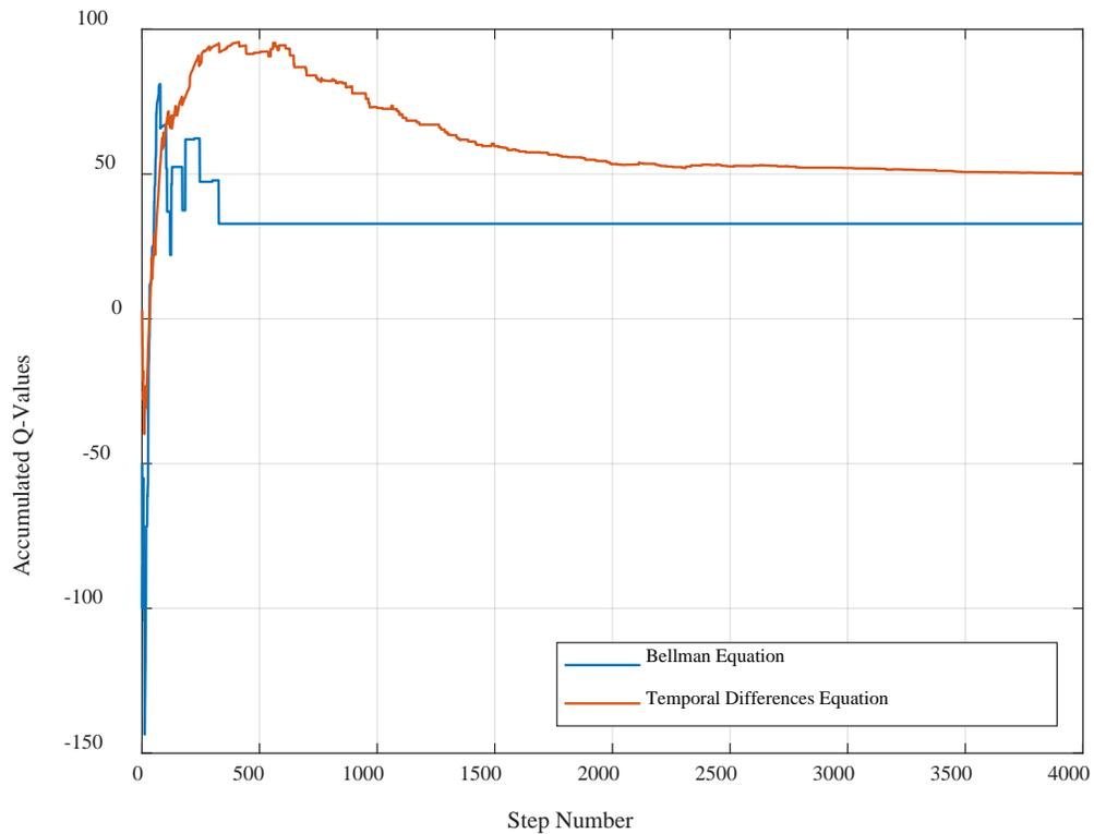
**Figure 27. Q-Matrix convergence: Bellman vs. TD equation.**
