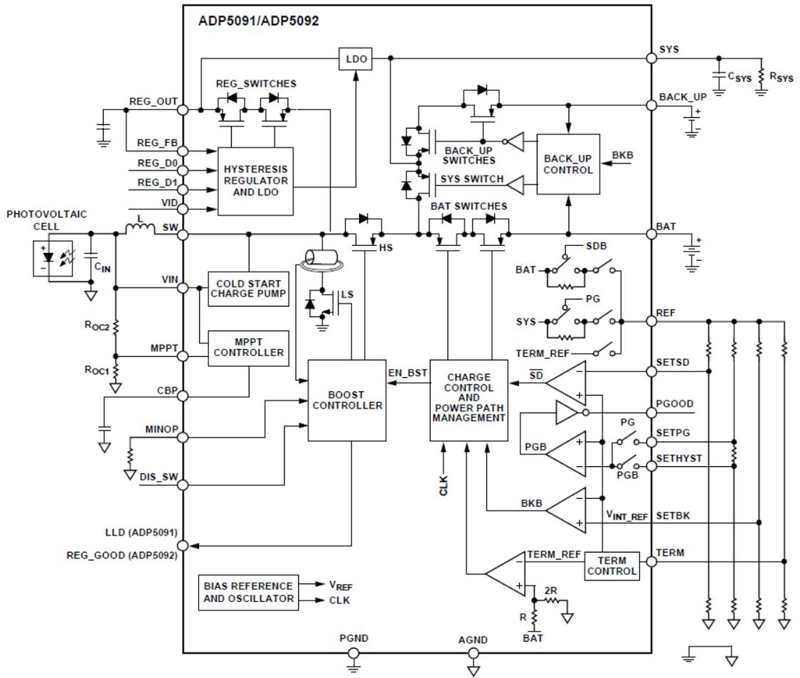
Figure 7. ADP5091 detailed functional block diagram [33].
