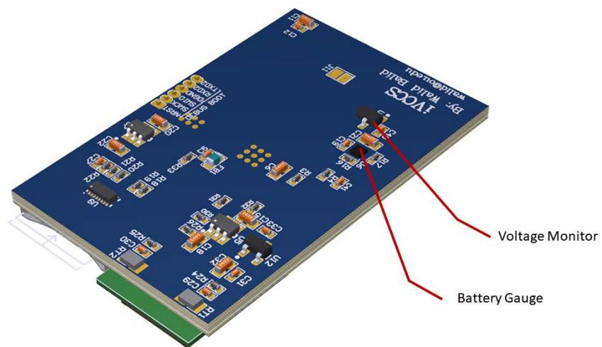
**Figure 5. *iVCCS* PCB components.**
