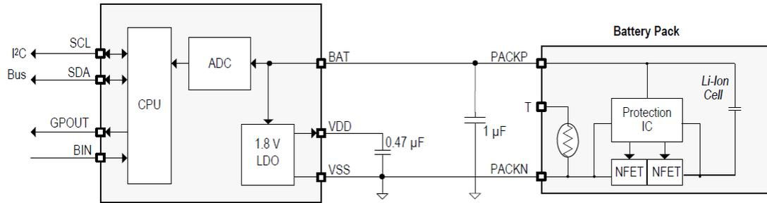
**Figure 6. Simplified schematic of the battery gauge unit [32].**
