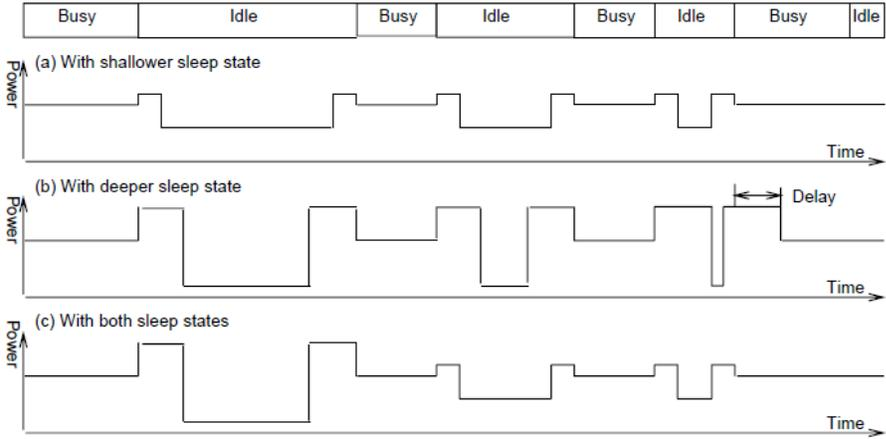
**Figure 3. Changing system sleep mode according to load [21].**
