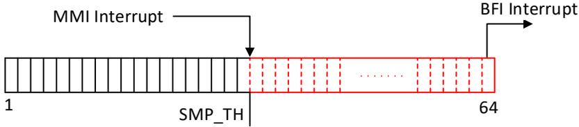
**Figure 18. MMI and BFI operation in KMX62 magnetometer.**
